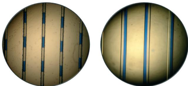
**Fig. 4.** Microscopic observation of the flow pattern formation in microreactor with rough and smooth channel walls (blue – aqueous phase, colorless – organic phase)
