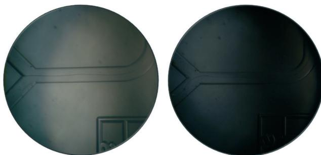
**Fig. 5.** Microscopic observation of the flow patterns at the exit of the microchannel for the flow ratio of aqueous and organic phase 1:3 and 1:1
