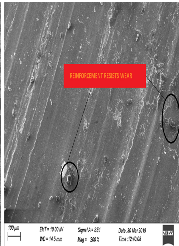
Fig. 8.b Worn surface of AL7075-12%TiB 2 -4.5%MoS 2
