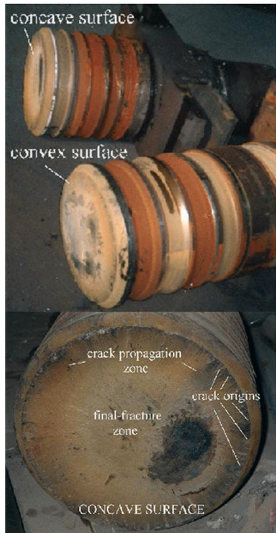
Fig. 4. Fracture surfaces of the 1<sup>st</sup> broken roll and the position of the stocks at the time of the fracture
