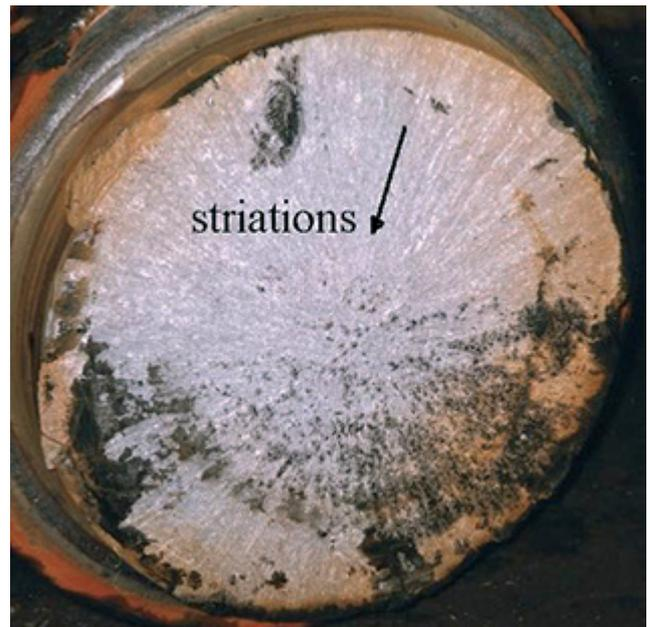
Fig. 6. Fracture surfaces of the 3<sup>rd</sup> broken roll and the position of the stocks at the time of the fracture
