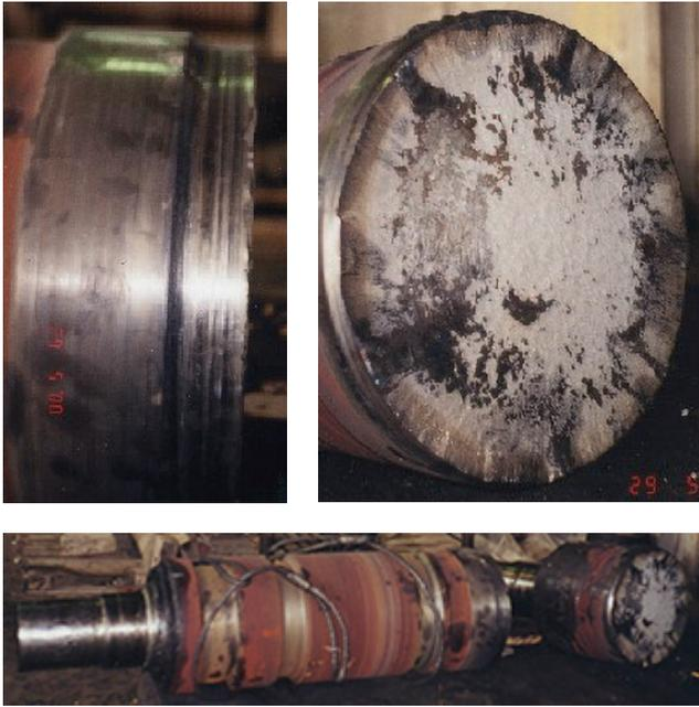
Fig. 7. Fracture surfaces of the 4<sup>th</sup> broken roll and the position of the stocks at time of the fracture
