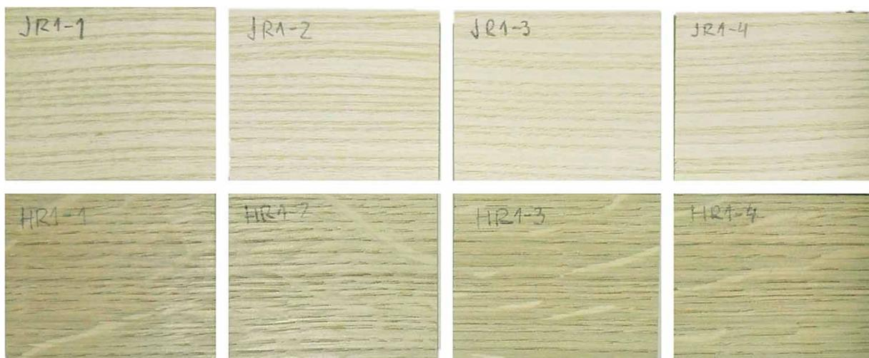
**Figure 1** Parallel specimens of ash (top) and oak (bottom) for drying at temperatures of 60 °C (1-1), 70 °C (1-2), 80 °C (1-3) and 90 °C (1-4)
