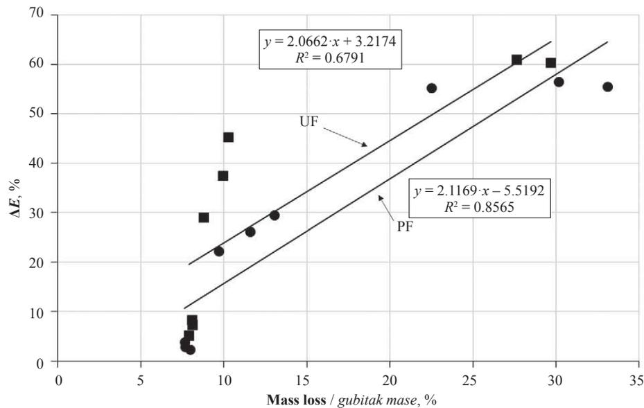
**Figure 1** Correlation between total colour difference and mass loss of samples
