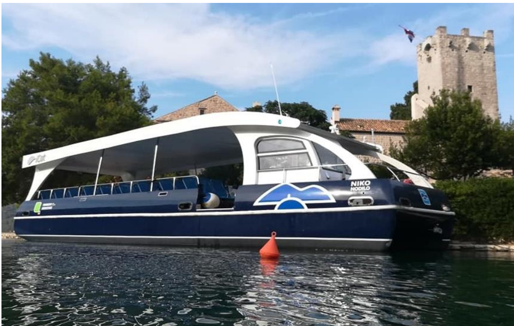
Fig. 10 Solar Powered Passenger Ferry (babyCat1) in service in Mljet National Park
