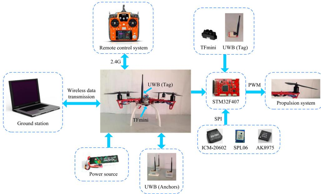
Figure 17. Experimental equipments of quadrotor UAV.
