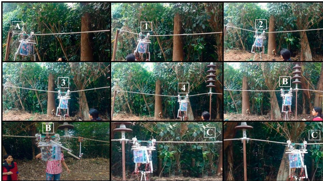
Figure 33. Testing of robot traversing on the straight transmission line: Snapshots.
