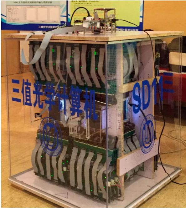
**Figure 5.** SD11 experimental system.
