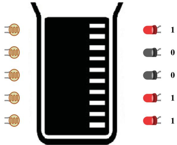
**Figure 9.** Decimal representation of combination of LEDs using binary. (e.g. Combination 25 means taking 1st, 2nd and 5th LDR sensors’ data from bottom to top into calculations like they are on, and excluding data of 3<sup>rd</sup> and 4th LDRs like they are off. Decimal representation of the combination above: 11001 = 25).
