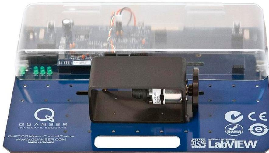
Figure 6. QNET DC motor control trainer.
