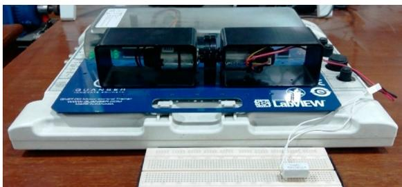
Figure 11. Motor-generator coupling to analyse load–torque variations.
