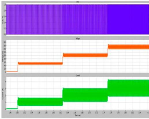
**Figure 12.** PWM wave of the converter; unipolar output from the converter; load current variation.
