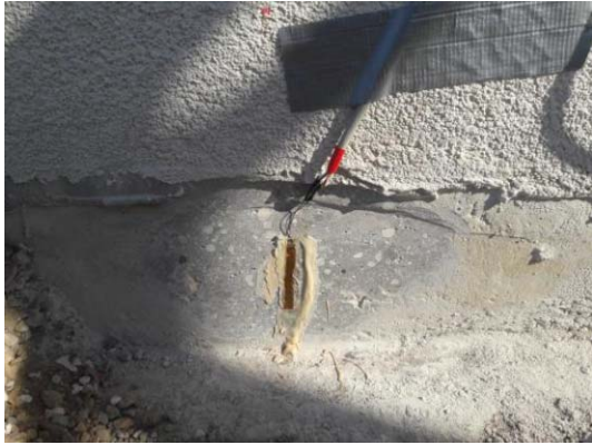
Figure 10. Measurement of strains at the base of the RC arch
