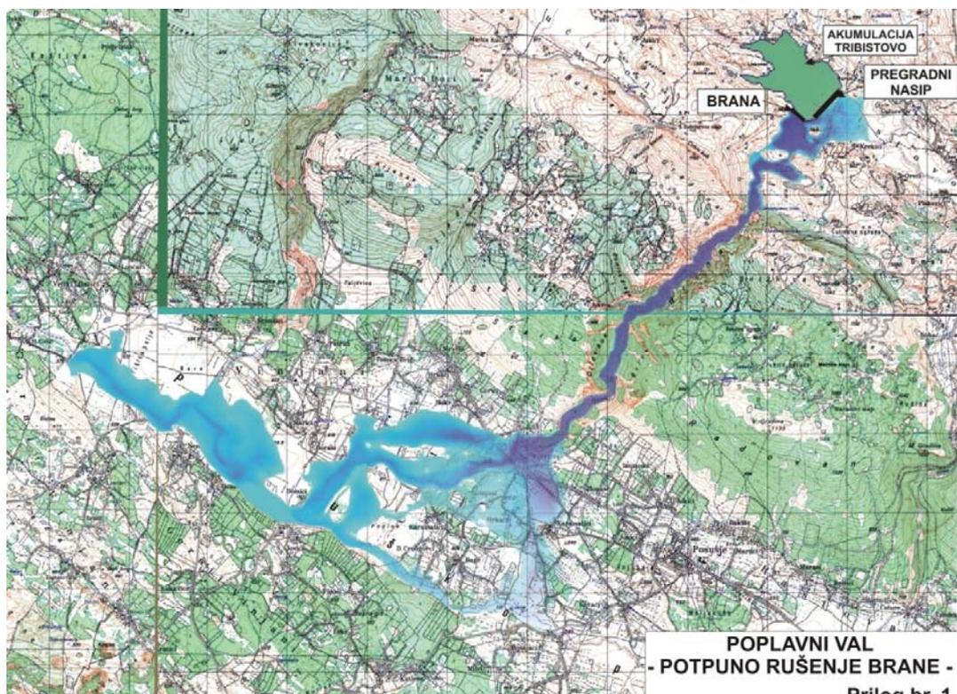
Figure 6. Flood hazard map for instantaneous and complete break of the dam
