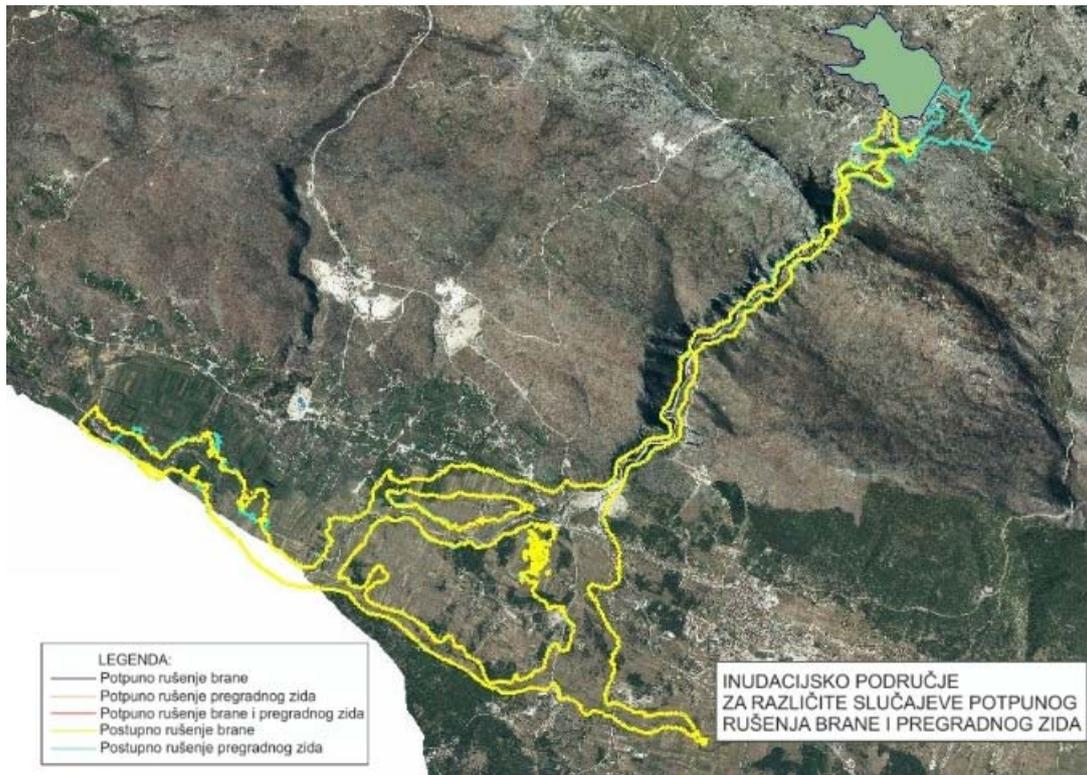
Figure 5. Limits of the flood waves from the hydraulic model for different dam and barrier embankment failure scenarios
