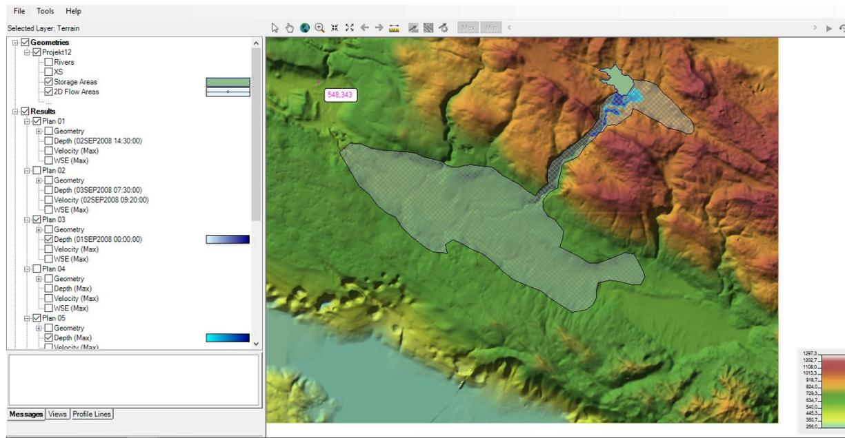
Figure 4. Calculation results with generated 2D calculation mesh of the model area
