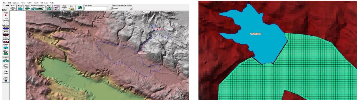
Figure 3. Left: map of the area with generated calculation mesh of the 2D model area; right: detail of the reservoir with the generated calculation mesh
