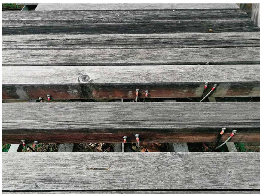
**Figure 2** Distribution of moisture content sensors in each layer of tested samples
