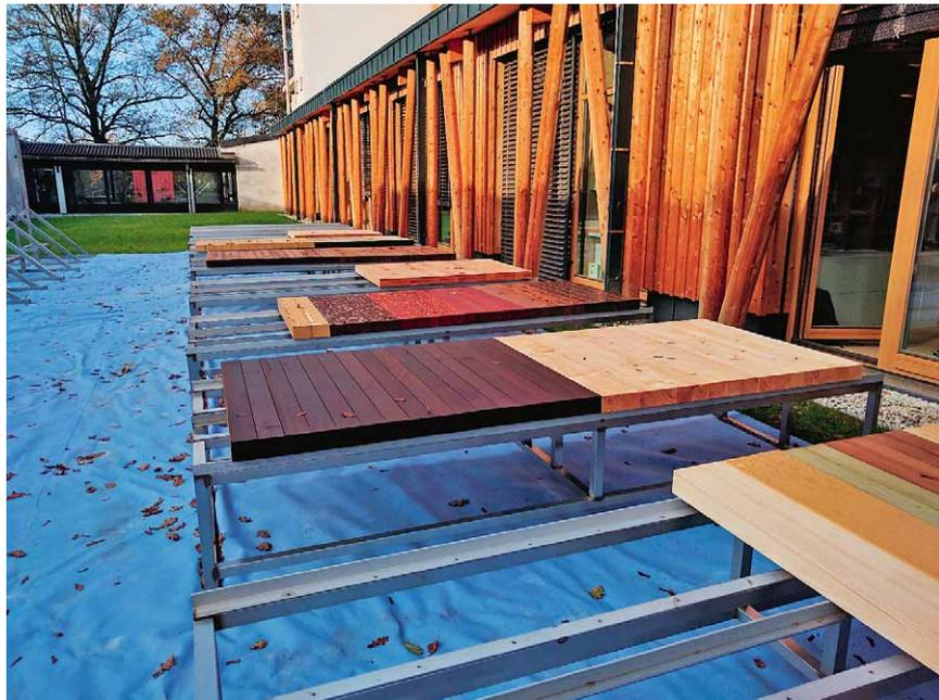
**Figure 1** Glulams at the beginning of the experiment on the test field of the University of Ljubljana, Biotechnical faculty
