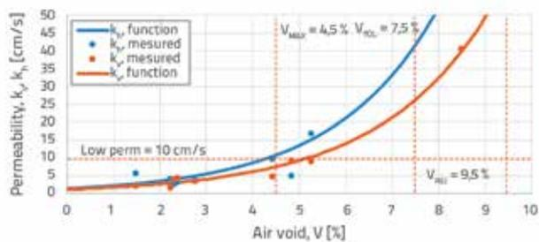
Figure 6. Measured and calculated permeability, SMA8 layer
