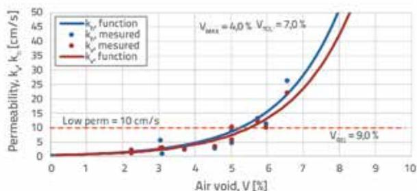
Figure 5. Measured and calculated permeability, AC11 layer
