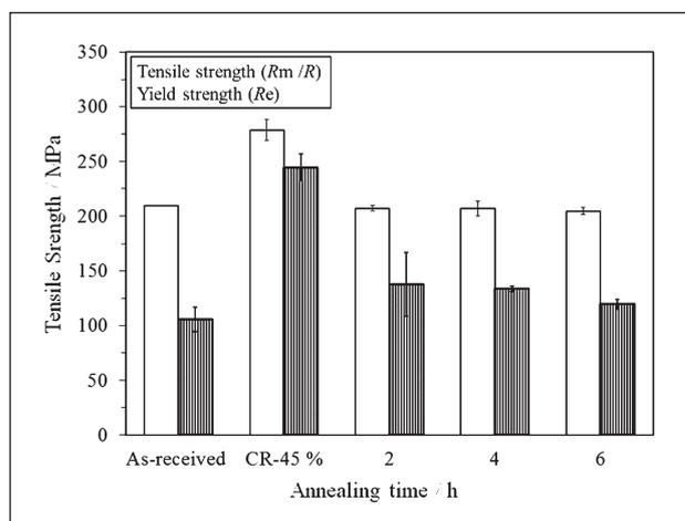
**Figure 7** Variation of yield and tensile strength with different annealing time
