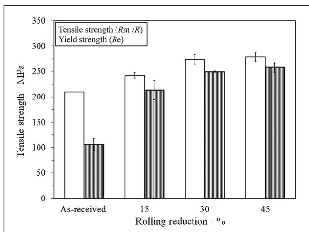
**Figure 5** Variation of yield and tensile strength with different rolling reduction
