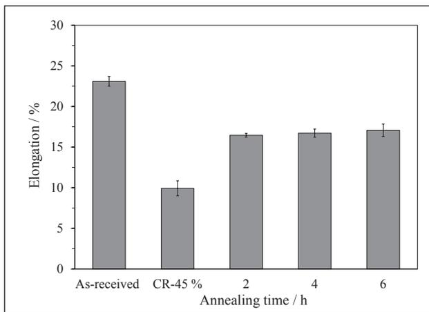
**Figure 8** Variation of elongation with different annealing time
