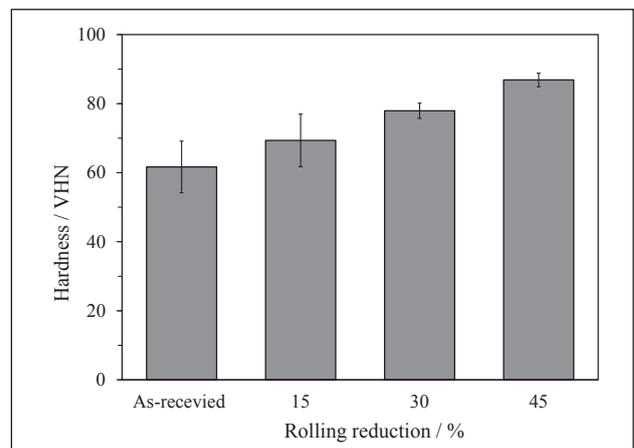
**Figure 3** Variation of hardness with different rolling reduction
