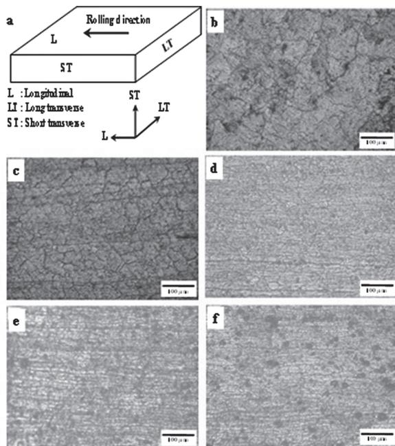
**Figure 1** (a) Three main directions in AA 5052 sheet with corresponding microstructures: (b) As-received sample in longitudinal direction (c) As-received sample (d) 15 % reduction rolled sample (e) 30 % reduction rolled sample (f) 45 % reduction rolled sample
