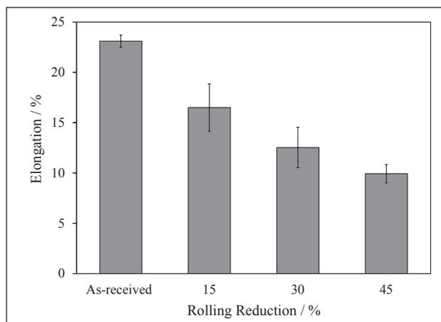
**Figure 6** Variation of elongation with different rolling reduction
