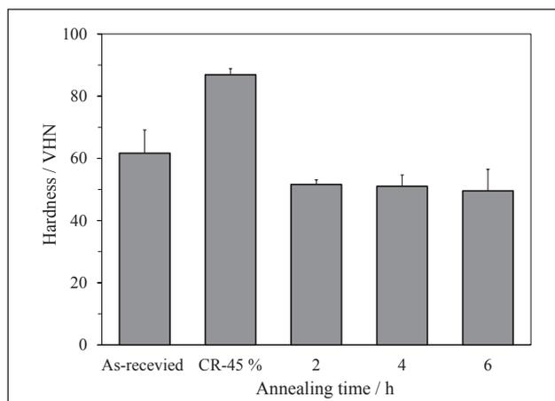
**Figure 4** Variation of hardness with different annealing time
