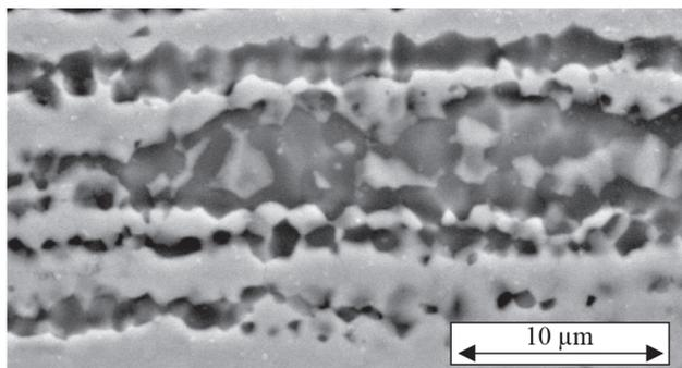
**Figure 4** SEM analysis of the longitudinal section of Zn-Al15 wire rod after 6 hours of heat treatment at 240 °C
