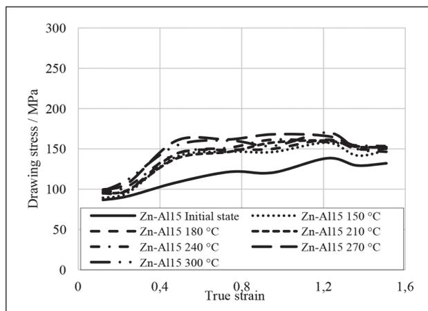
**Figure 6** Drawing stress values of Zn-Al15 wires after 6 hours of heat treatment at the selected temperatures from 150 °C to 300 °C with a sample at initial state as a reference material
