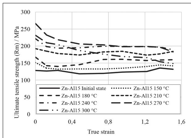
**Figure 7**  $R_m$  values of Zn-Al15 wires after 6 hours of heat treatment at the selected temperatures from 150 °C to 300 °C with a sample at initial state as a reference material
