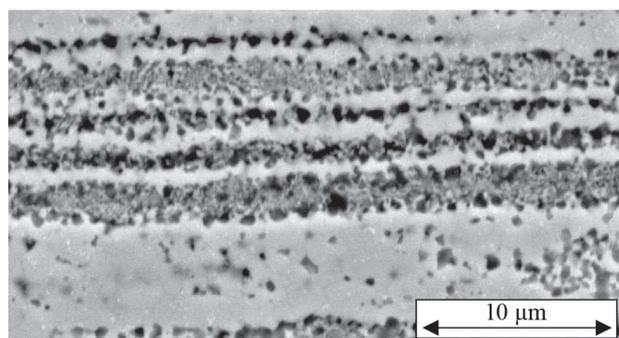
Figure 2 SEM analysis of the longitudinal section of Zn-Al15 wire rod at the initial state
