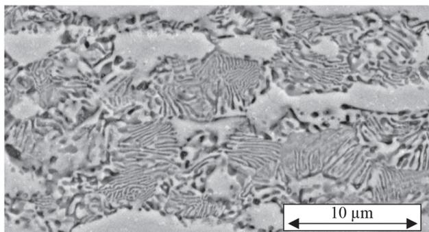
**Figure 5** SEM analysis of the longitudinal section of Zn-Al15 wire rod after 6 hours of heat treatment at 300 °C
