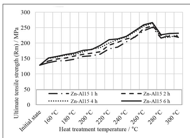
Figure 1  $R_m$  values of Zn-Al15 wire rod after heat treatment at the temperatures from 150 °C to 300 °C with a sample at initial state as a reference material
