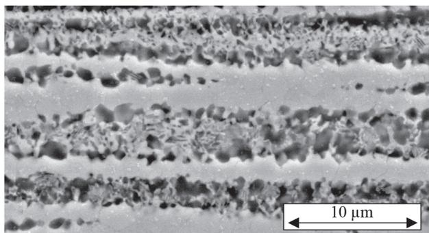
**Figure 3** SEM analysis of the longitudinal section of Zn-Al15 wire rod after 6 hours of heat treatment at 180 °C
