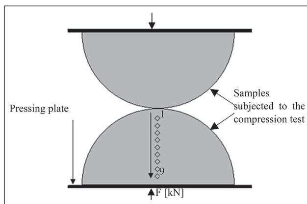
**Figure 1** Compression test of the aluminum alloy samples with the marked places of the later indentations (1 – 9) which were made during Vickers hardness test
