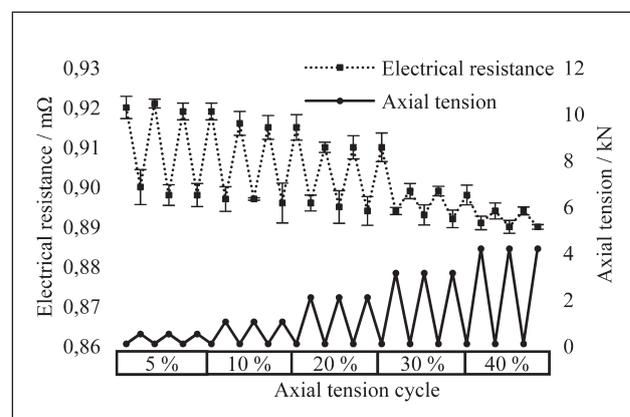
**Figure 2** The influence of the axial tension on the electrical resistance OHL conductor with standard deviation marked as error bars
