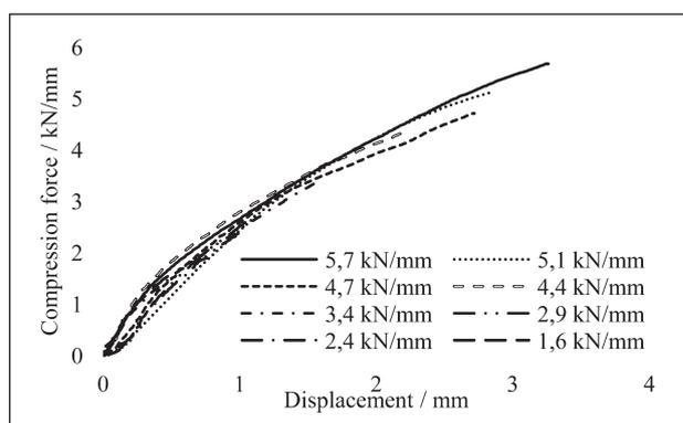
**Figure 3** Compression force in the function of displacement with the maximum force of 50 kN (5,7 kN/mm)
