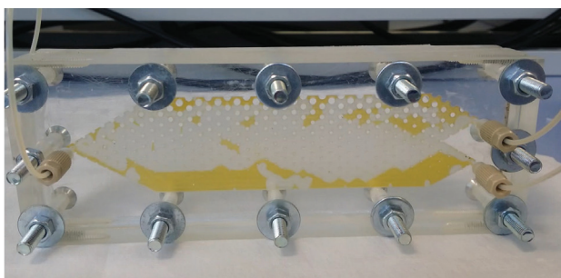
Fig. 3 – External view of the initial microseparator geometry: single inlet is on the left-hand side whereas two outlets (one for each phase) are on the right-hand side of the picture.
