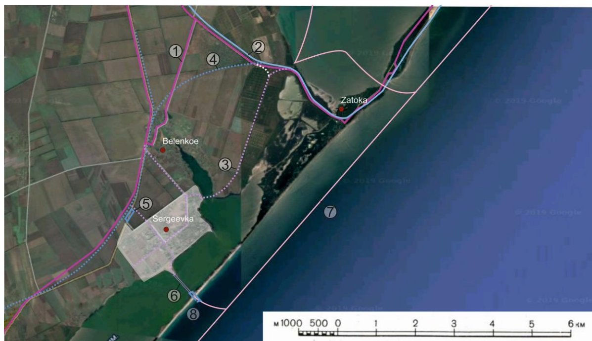
Figure 7 Organizational concept of the transport system of Sergeevka resort: 1) existing highway; 2) existing railway; 3) proposed highway; 4) proposed railway; 5) and transport hub. 6) Renewed pedestrian-transport bridge integrated into the urban transport and pedestrian scheme. 7) Renewable water-transport concept and 8) the proposed seaport with leisure facilities year-round. [20]
