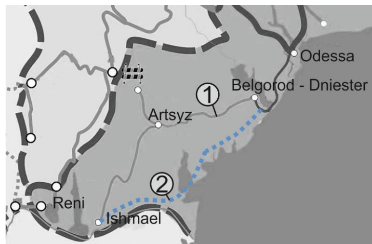
Figure 6 Organizational scheme of Sergeevka railway communitie: 1) existing railway line and 2) proposed railway line along the coastline.
