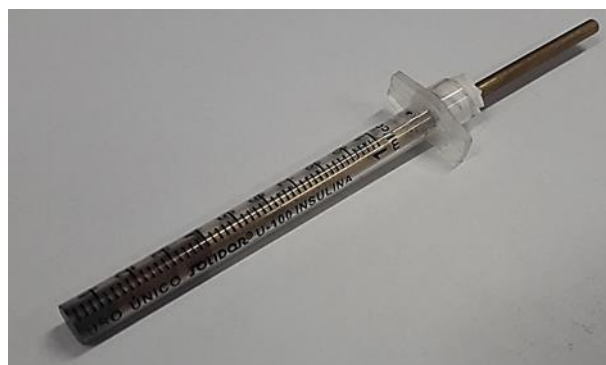
Figure 2. Carbon paste electrode prepared and employed in this research
