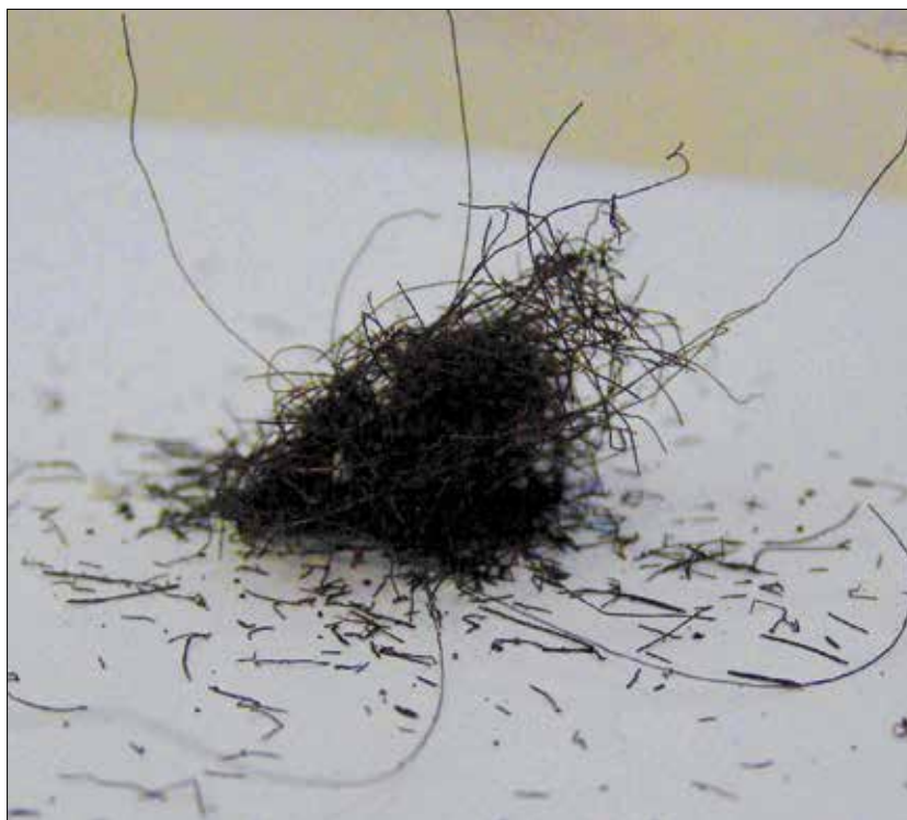
Figure 6. Disintegrated copper due to corrosion
