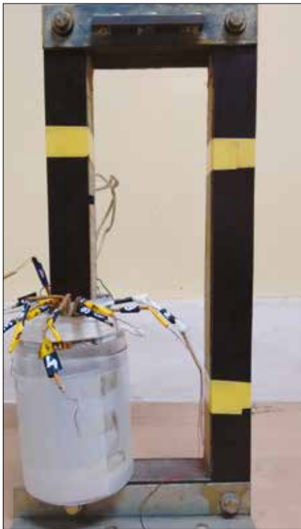
Figure 4a. 10 section multi-layer winding
