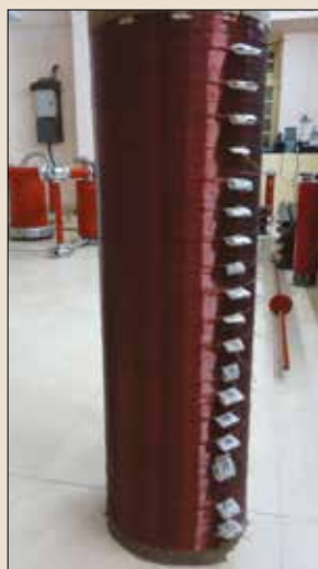
Figure 1a. Single-layer winding
