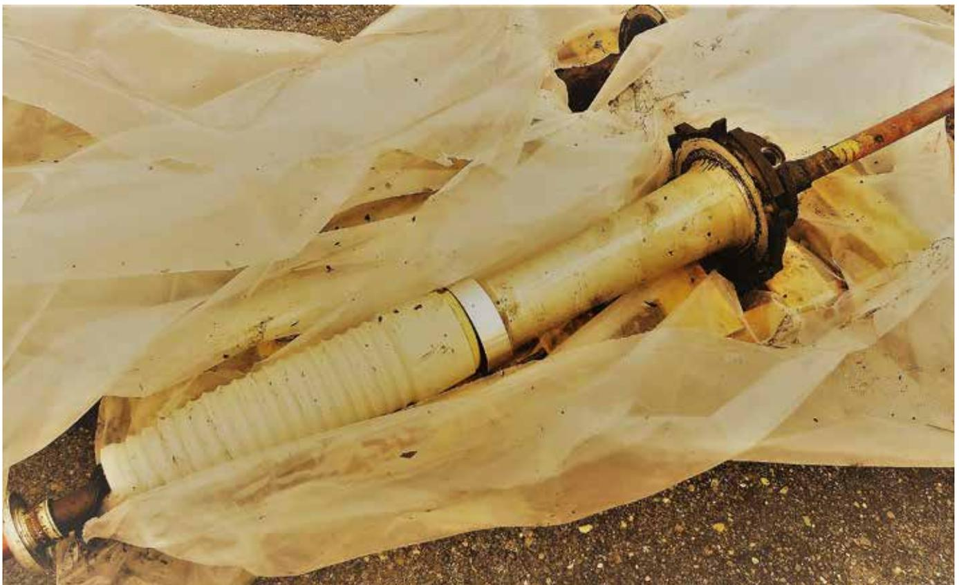
Figure 3. Investigated ABB, 69 kV, type O+C bushing failure for case study 2
