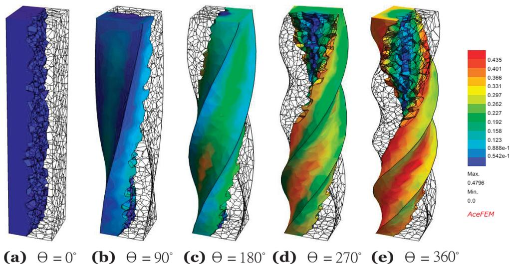
**Fig. 6.** Numerical torsion test of a square-section bar. Distribution of the equivalent plastic strain  $\bar{\epsilon}$  for different rotations angles until the cycle is completed using the VEM-VO element.
