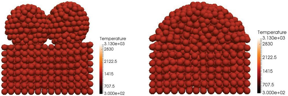
**Fig. 15.** Melting and solidification of two laser-irradiated particles using the stabilized OTM method, (left) neglecting and (right) including the surface tension effect.
