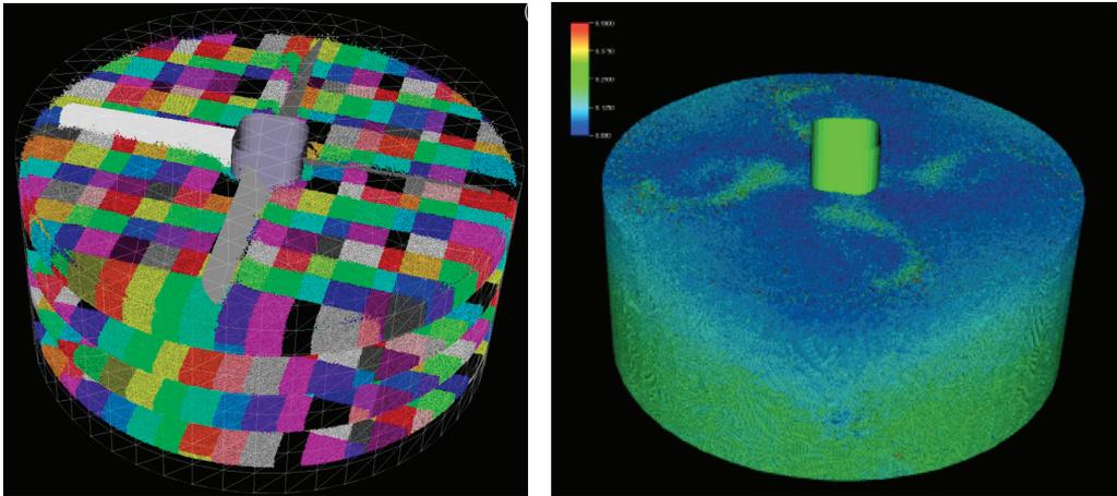
**Fig. 10.** a) Set-up of the particles in the mixer. The color code shows the allocation to a core in the parallel computer. b) Velocity distribution of the particles during mixing.
