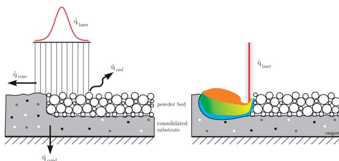
**Fig. 14.** (Left) Laser irradiation is emitted by thermal conduction, convection and radiation. (Right) Melt pool due to molten particles.
