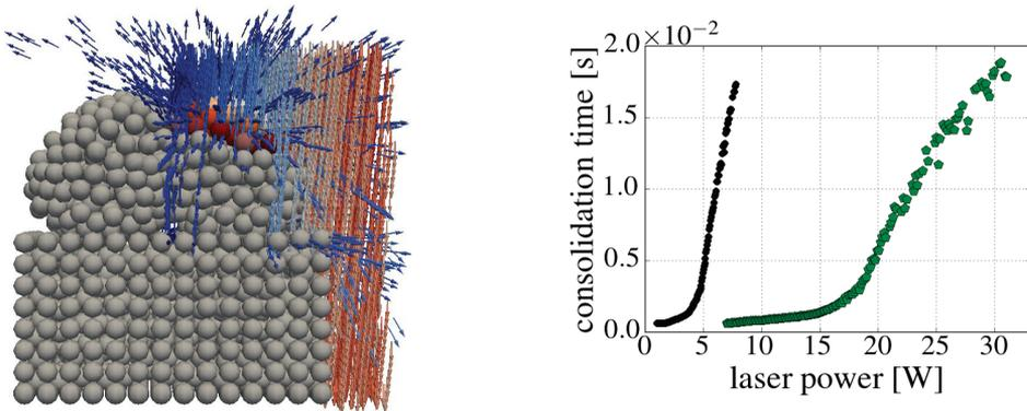
**Fig. 16.** (Left) Ray tracing approach coupled with the stabilized OTM method. (Right) Comparison of consolidation time between volumetric heat source model of [9] (green dots) and ray tracing approach (black circles).
