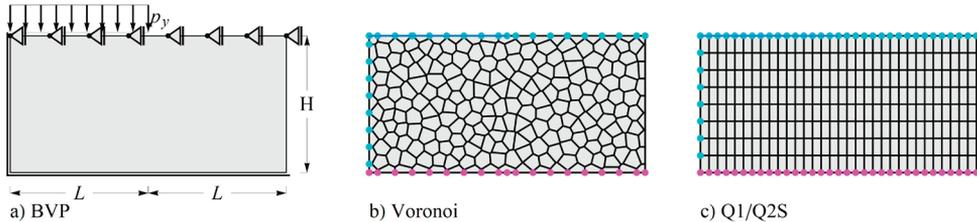
**Fig. 3.** Punch problem and different mesh types.
