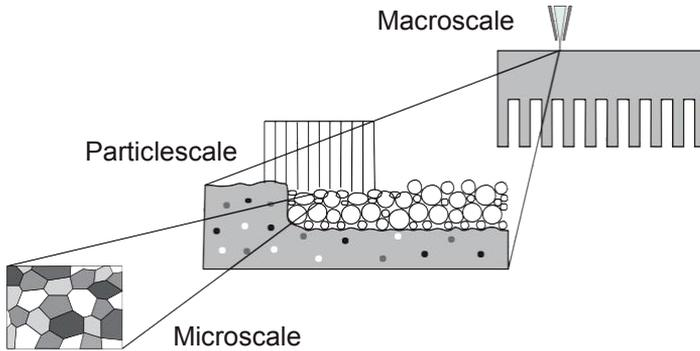
**Fig. 20.** Multiscale approach for modeling additive manufacturing processes.
