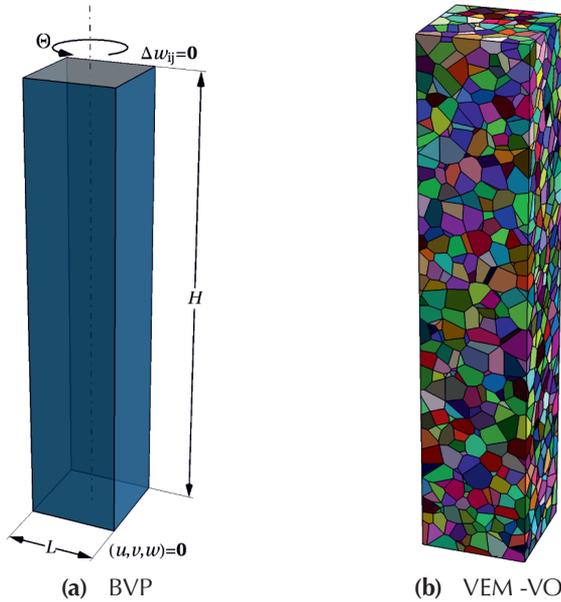
**Fig. 5.** Numerical torsion test of a square-section bar. (a) Geometry and boundary conditions; (b) Voronoi mesh used in the numerical analysis for  $9 \times 9 \times 36$  elements.
