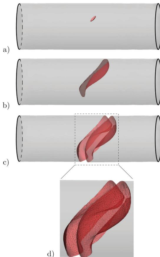
**Fig. 7.** Three-dimensional torsion test of a cylindrical bar. (a)–(c) Contour plots of the fracture phase-field  $d$  evolution in brittle (Elastic-Fracture) cast-iron for a twist loading. (d) Visualization of the crack faces.
