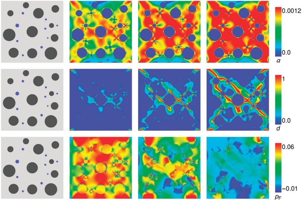
**Fig. 9.** Compression test for idealized microstructure of concrete specimen under water. Dark gray circles represent the stones, blue circles stand for water (saturated voids), and the rest with light gray color stands for the cement paste (mixture). Evolution of the hardening variable  $\alpha$ , crack phase-field  $d$  and fluid pressure  $p_F$ .
