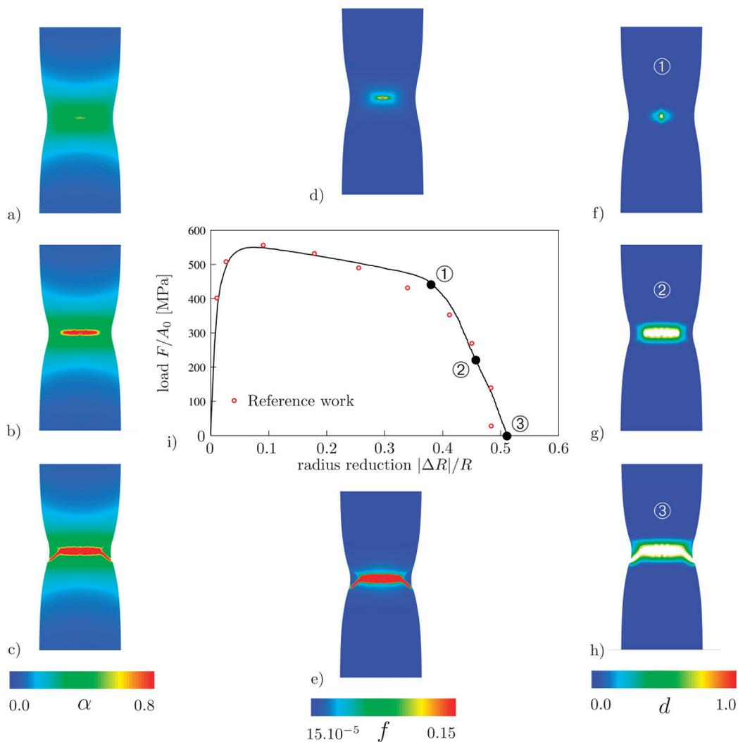
**Fig. 8.** Cup–cone formation in axis-symmetric tension test. Contour plots of the hardening variable  $\alpha$  in (a)-(c); the void volume fraction  $f$  in (d)-(e) and the fracture phase-field  $d$  in (f)-(h). Load (force  $F$  / initial cross sectional area  $A_0$ ) versus magnitude of the radius reduction  $|\Delta R|/R$  curve in comparison with the reference work of Besson et al. [2001] is shown in (i).
