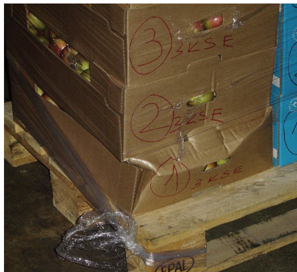
Image 2 Corrugated cardboard boxes with lower technical parameters
