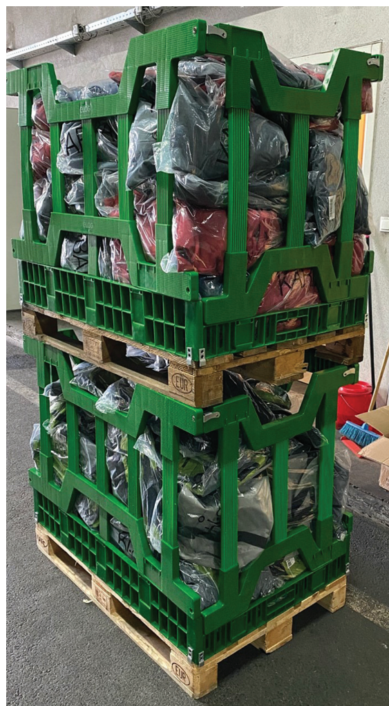
Image 9 X-Bin – the option of vertical stacking of transport units
