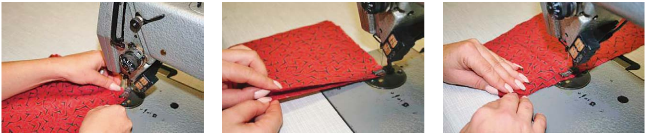
Fig.6 Representation of the sequence of motions for the method of individual work piece guiding
