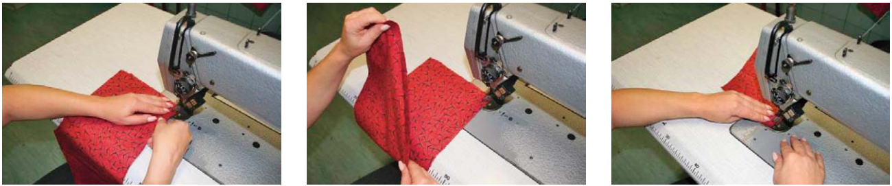
Fig.5 Representation of the sequence of motions for the basic guiding method with two control points
