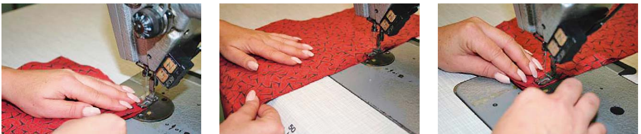
Fig.3 Representation of the sequence of motions using the method of joint guiding on the universal sewing machine
