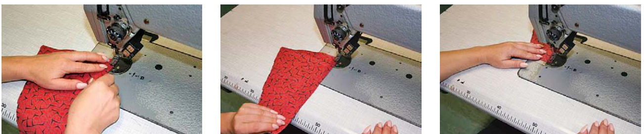
Fig.4 Representation of the sequence of motions with one control point
