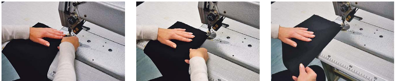
Fig.13 Representation of the sequence of motions to change the grip
