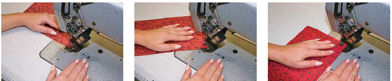
Fig.16 Representation of the sequence of motions for rotating the work piece around the needle with one hand
