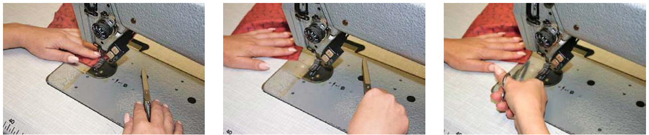
Fig.11 Representation of the sequence of motions for cutting off the thread using normal scissors
