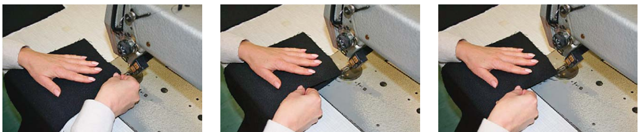
Fig.14 Representation of the set of motions for aligning the contour edges with changing the grip of the right hand
