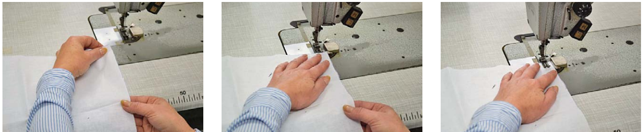
Fig.10 Representation of the sequence of positioning the work piece using the auxiliary device – ruler
