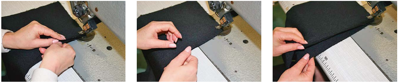
Fig.15 Representation of the set of motions for aligning the contour edges with changing the grip of both hands
