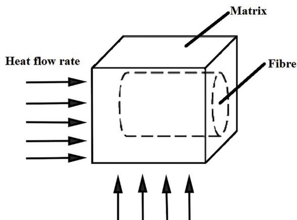
Figure 3 Effect of heat flow on a fiber of composite material
