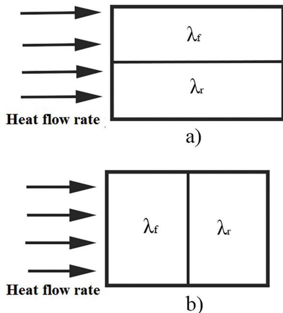
Figure 4 Parallel and vertical effect of heat flow on the matrix and composite reinforcement
