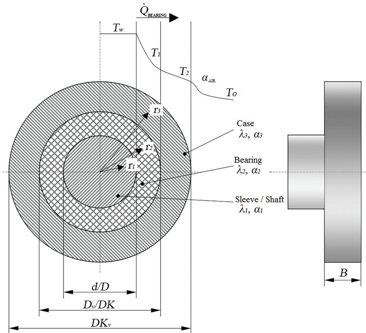
Figure 2 Thermodynamic model of the sliding bearing / sleeve system
