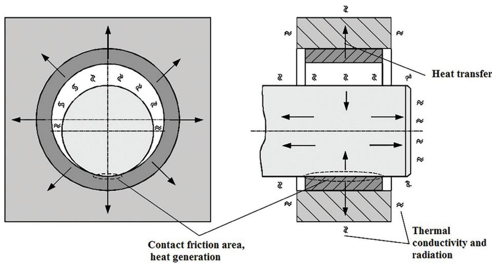
Figure 1 Heat generation in system bearing /sleeve
