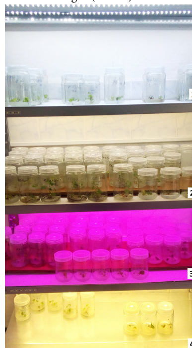
Figure 1. Photographs of the plantlets illuminated by the LED bars: 1 – cool white light (6000K); 2 – natural white light (4000K); 3 – 20% blue light with a wavelength of 460 nm and 80% red light at a wavelength of 660 nm; 4 – warm white light (2700K)
