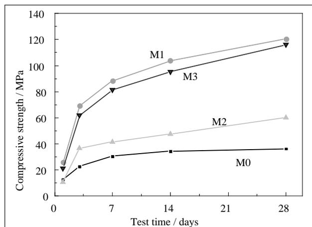
Figure 1 Compressive strength of MOS cement
