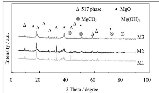
Figure 4 XRD patterns of modified MOS cement with different molar ratios
