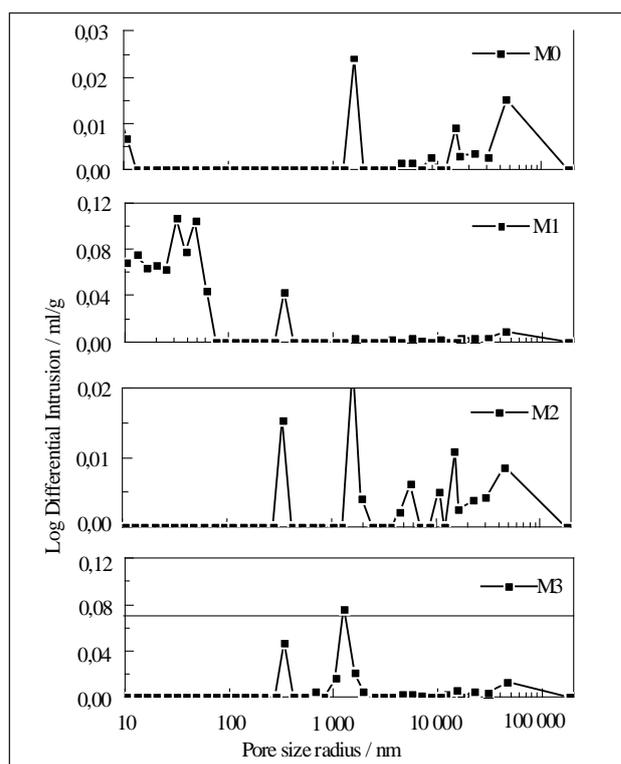
Figure 2 Differential pore distribution curve of MOS cement
