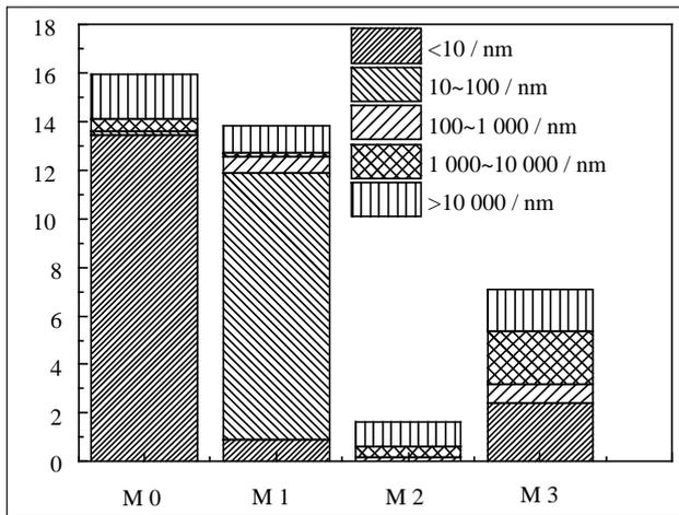
Figure 3 Porosity and pore distribution of MOS cement pastes
