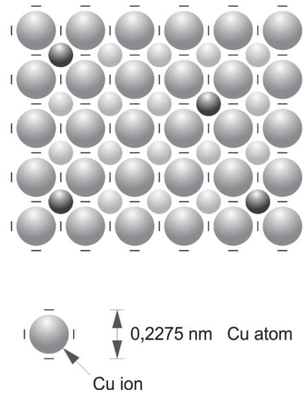
**Figure 1** Segment of wire cross section with apparent sections of copper atoms, ions and interstitial quanta-paths (pq), some with oxygen atoms. The calculated section of atom lattice space is marked with 4 dashes representing 4 FE vibration amplitude planes.
