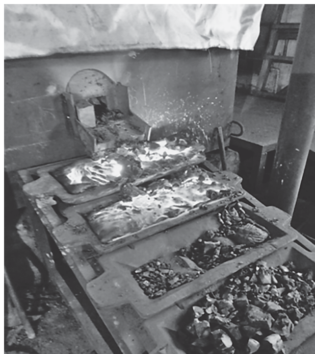
Figure 1 Release of ferromanganese from the 0,3 MVA furnace
