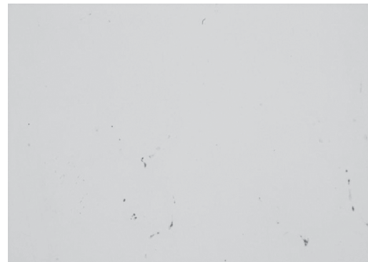
Figure 4 Experimental casting contamination with non-metallic inclusions, ×500
