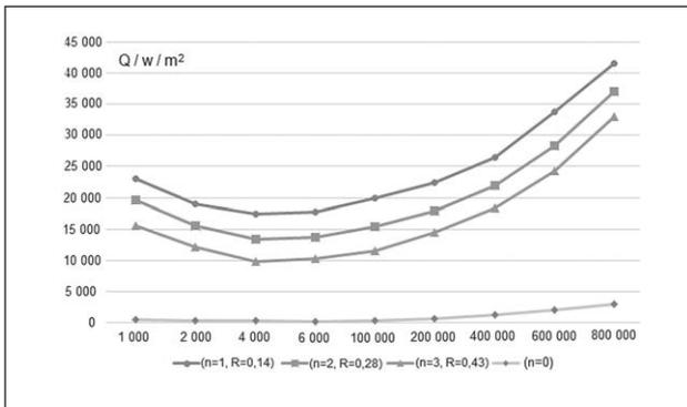
**Figure 2** Dependence of the removed heat flux  $Q/W/m^2$  on the heat flux density  $q/W/m^2$  at different layers.
