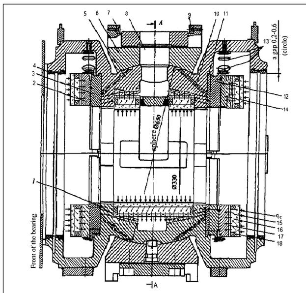
1-drilling; 2, 4, 12-setting rings; 3-resistant segment; 5-liner; 6-holder; 7,9-rings; 8-channel; 10-drilling; 11-spacer; 12-plate; 13-vent; 14-feather; 15-vapor stream; 16-adiabatic zone; 17-fluid flow; 18-capillary-porous structure;  $q_e$ ,  $q_c$  - heat flow in the evaporator and condenser.
