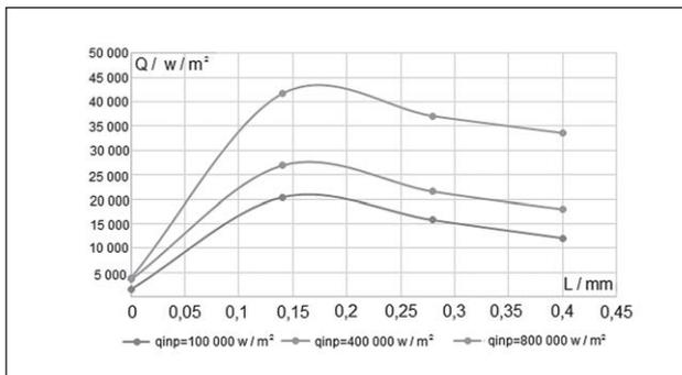
**Figure 3** Dependence of the removed heat flux  $Q/W/m^2$  on the cell size  $r, mm$  with one layer:  $m_w = (1 - 7,5) mm$ ; 1-structure 0,14; 2-structure 0,28; 3-structure 0,42
