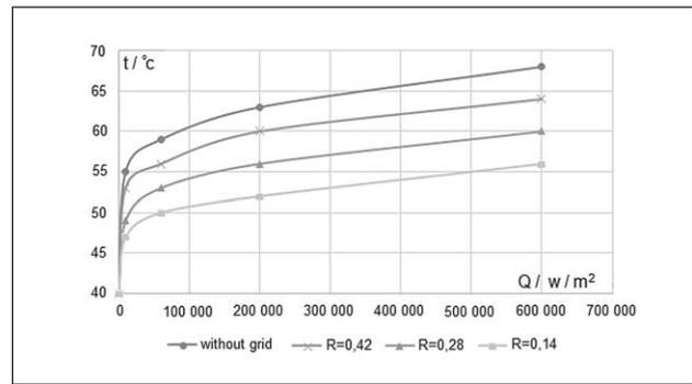
**Figure 4** Dependence of the oil temperature  $t/^\circ C$  from the heat flux density  $q/W/m^2$  for pressure  $P = 0,1 MPa$  for one layer.
