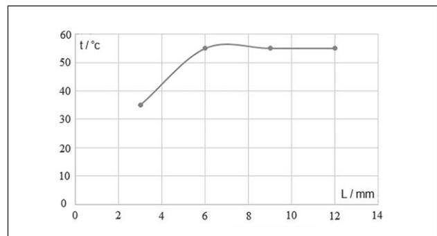
**Figure 5** Dependence of oil temperature  $t/^\circ C$  along the length of the bearing diameters  $L/mm$
