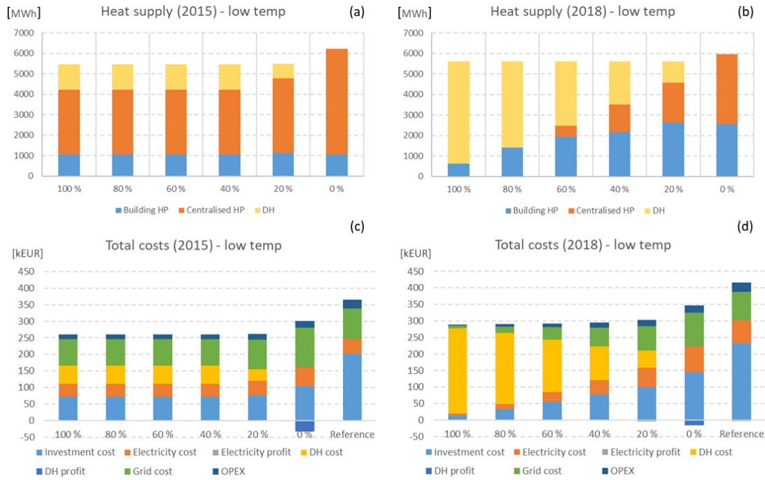
Figure 5. Heat supply (a-b) and total costs (c-d) of energy system in building area as a function of maximum share of DH supply in the case of low DH temperature
