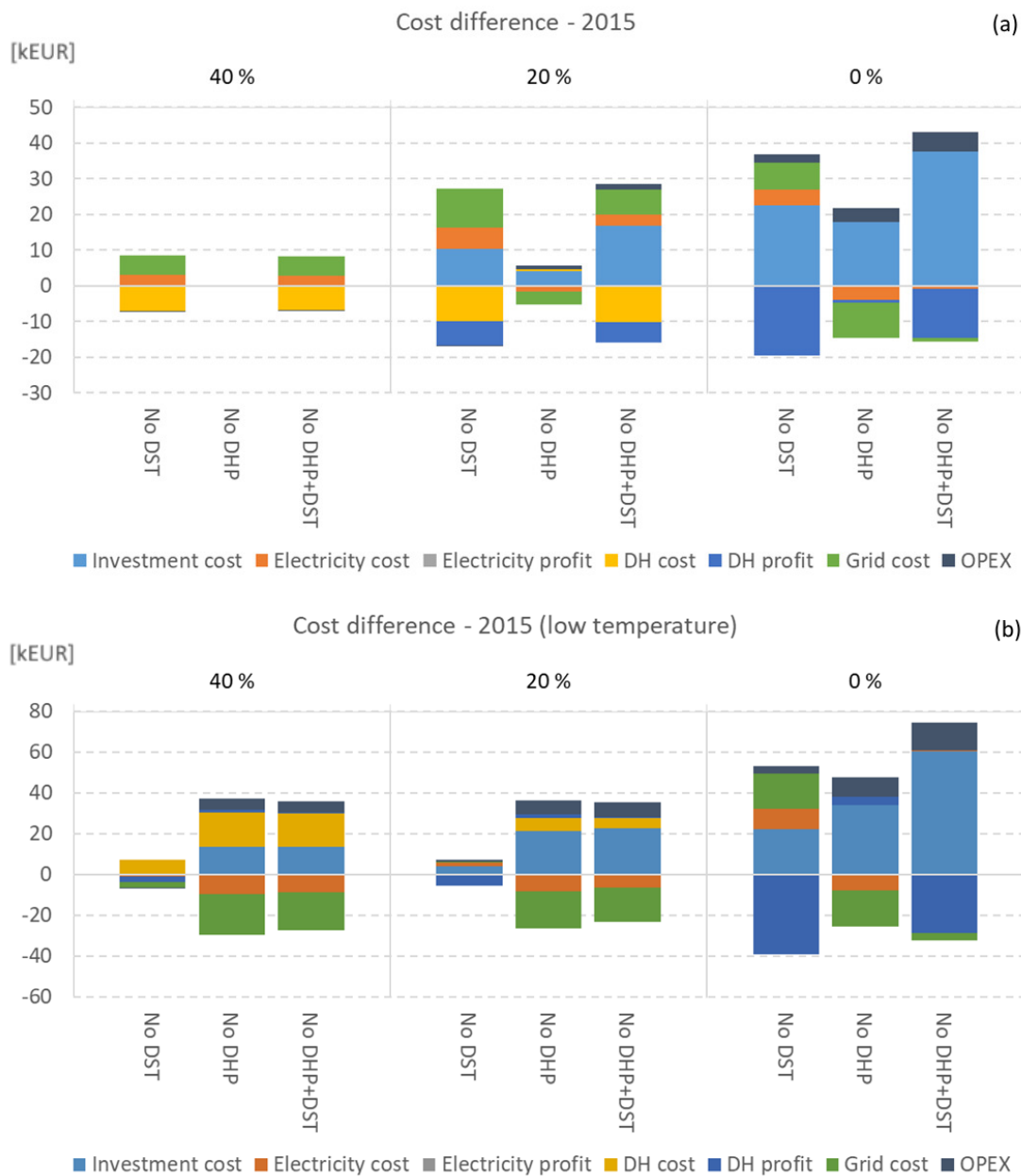
Figure 8. Difference in in total cost between regular case and cases with centralised heat storage removed ('No DST'), central ground HP removed ('No DHP') and both removed ('No DHP + DST') in year 2015 in the case of normal DH temperature (a) and low DH temperature (b)
