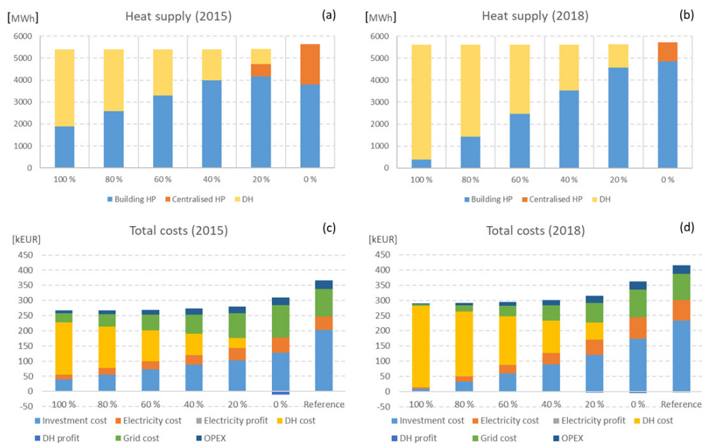
Figure 4. Heat supply (a-b) and total costs (c-d) of energy system in building area as a function of maximum share of DH supply in the case of normal DH temperature
