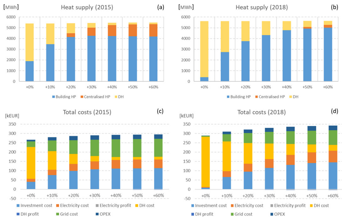
Figure 7. Heat supply (a-b) and total costs (c-d) of energy system in building area as a function of increase of DH supply price in the case of normal DH temperature
