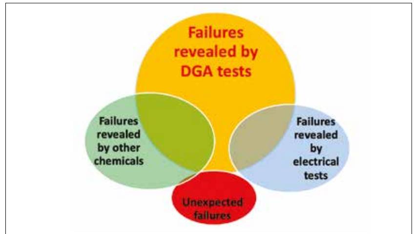
Figure 4. General concepts of the correlations between different measurement types and preventing failure probability for insulating power transformers
