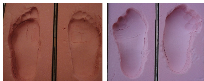
Figure 8 - 9: Imprint in PUR foam - deformed feet that create higher pressure than healthy feet
