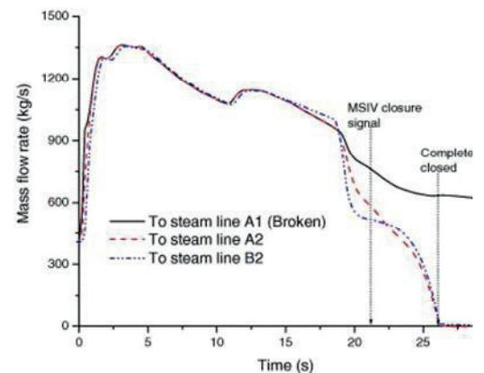
Figure 7: Steam line break outside of containment - steam flow rate at the steam generator exit, comparison with ref. [5]
