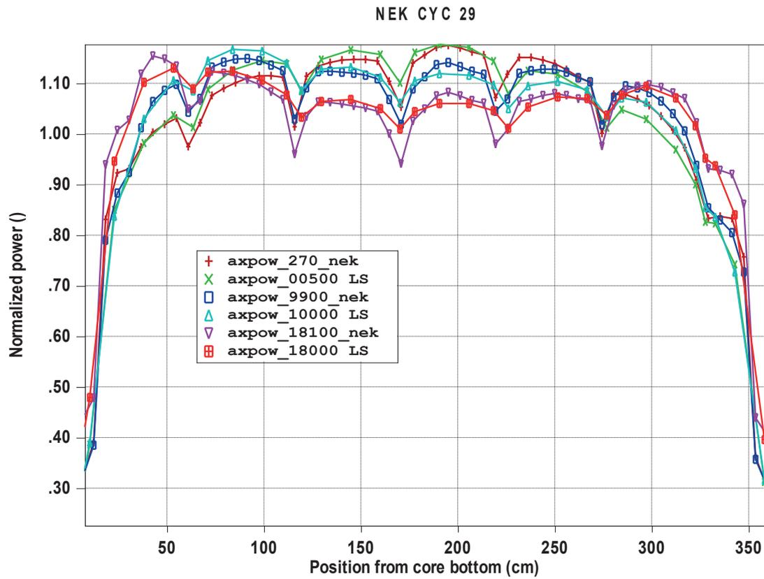
Figure 6 Comparison of axial power profiles with measured data at BOC, MOC and EOC
