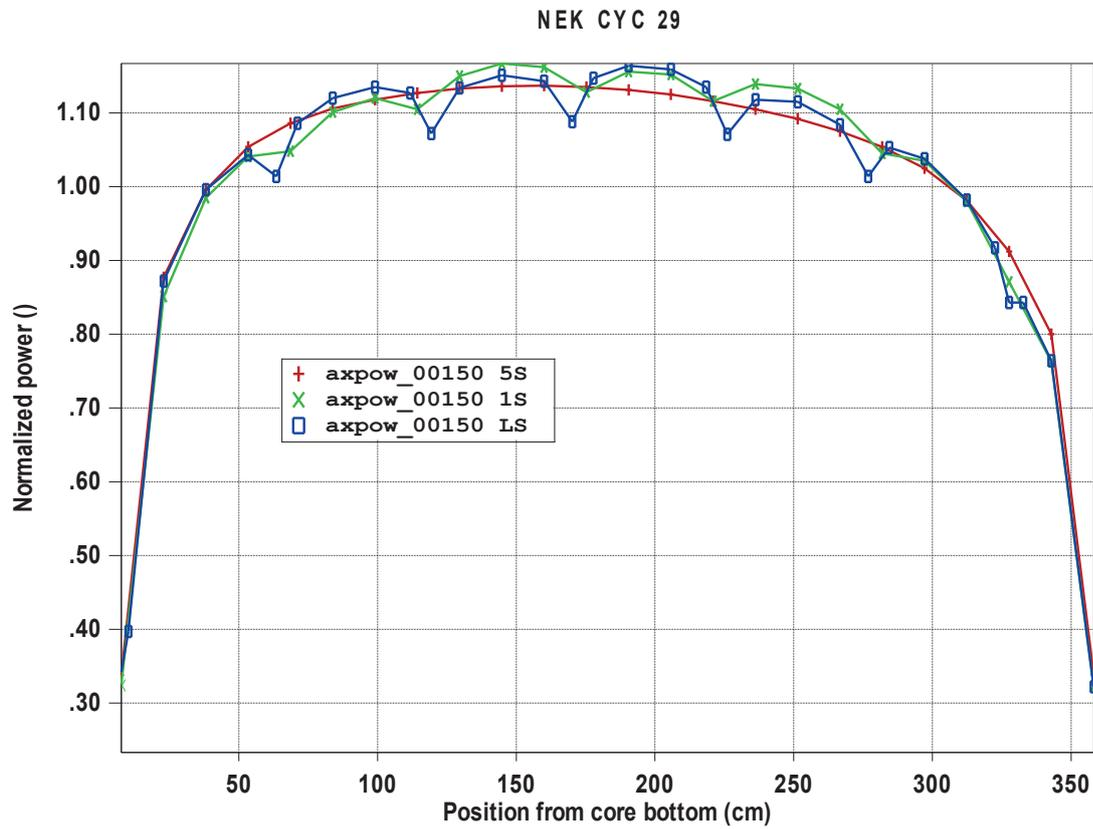
Figure 4 Axial power profile for three different ways of grids smearing - BOC
