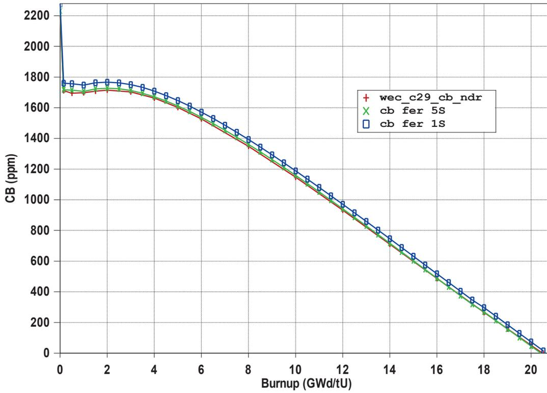
Figure 2 Influence of spacer grid homogenization on critical boron concentration
