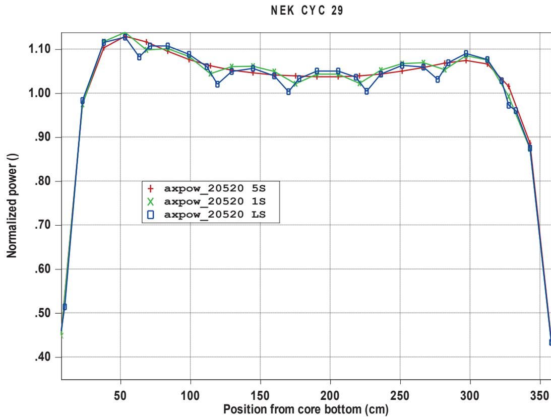
Figure 5 Axial power profile for three different ways of grids smearing - EOC
