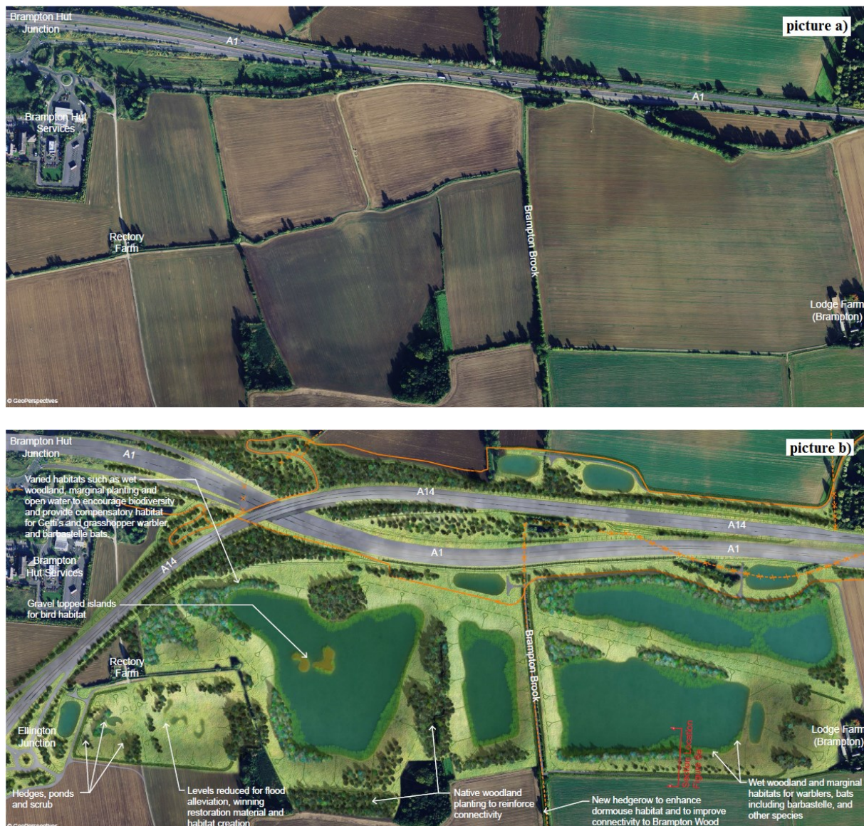
Figure 5. Borrow pit no. 1 (a – before exploitation, b – borrow pit design) (Highways England 2015)
