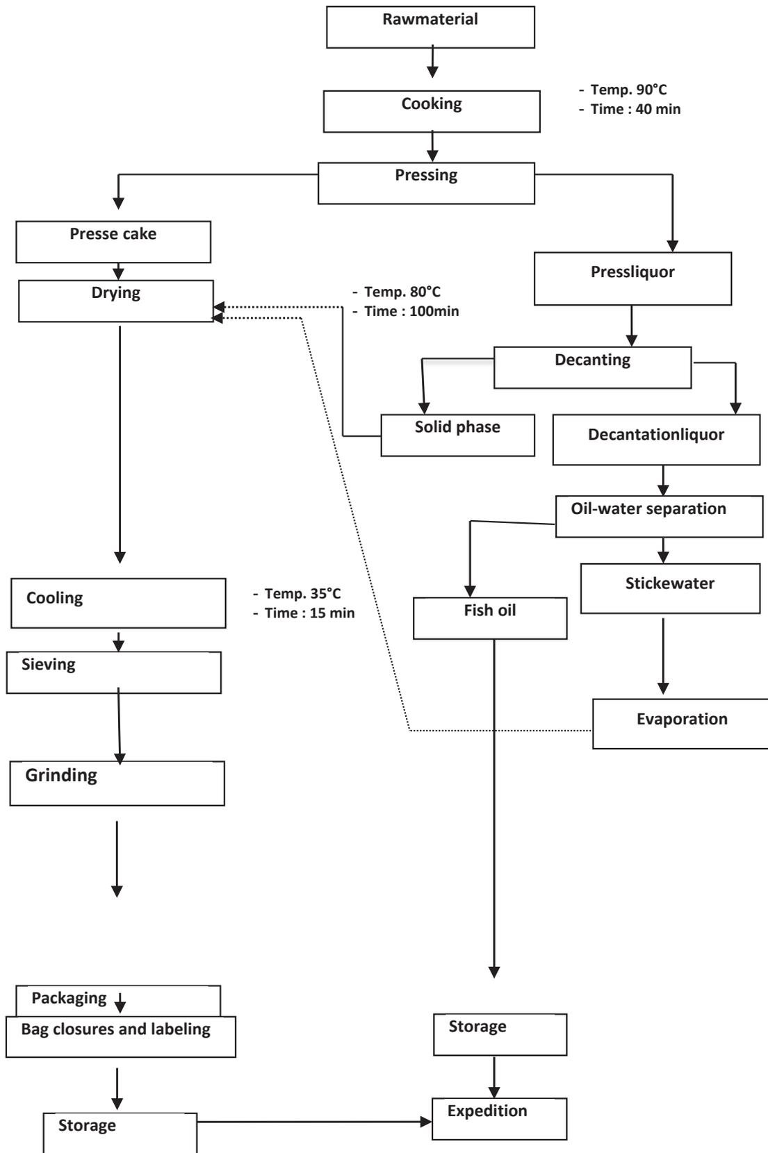
Fig 1. Stages and parameters of fish meal production
