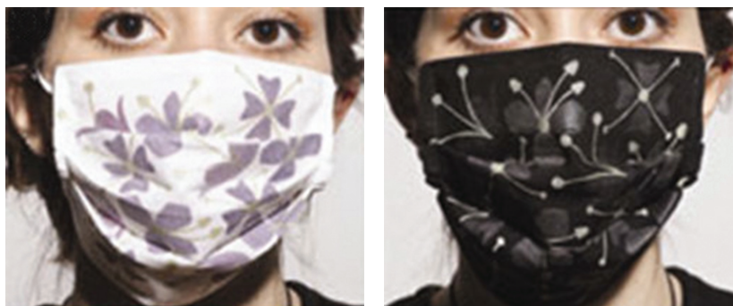
Figure 10. Colour change due to thermochromic print highlighting floral print on white background by changing from black colour when heat is supplied [22]
