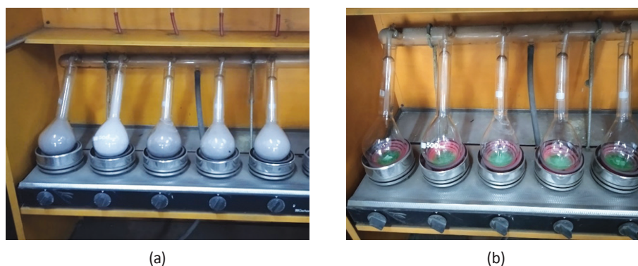
Figure 13. Digestion of raw trimmings (a) at the start of digestion and (b) at the end of digestion
