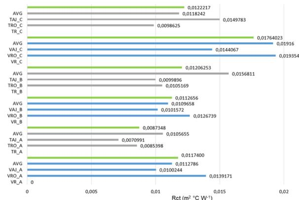
**Fig. 20** Thermal resistance of viscose and Tencel socks of group A, B, C
