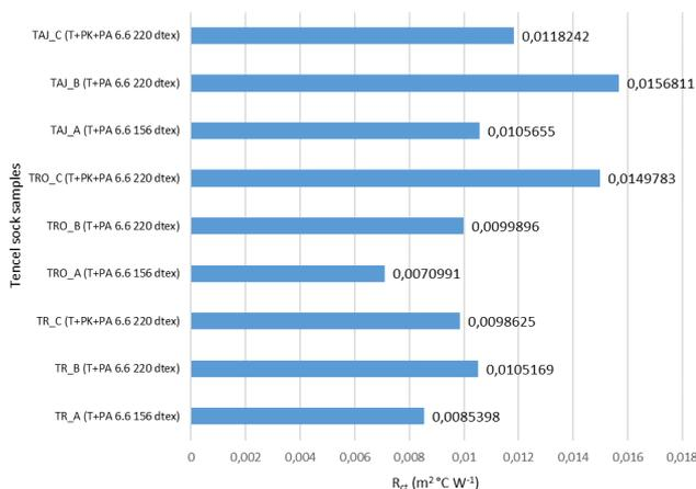
**Fig. 18** Thermal resistance of tencel sock samples
