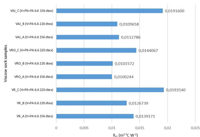
**Fig. 17** Thermal resistance of viscose sock samples
