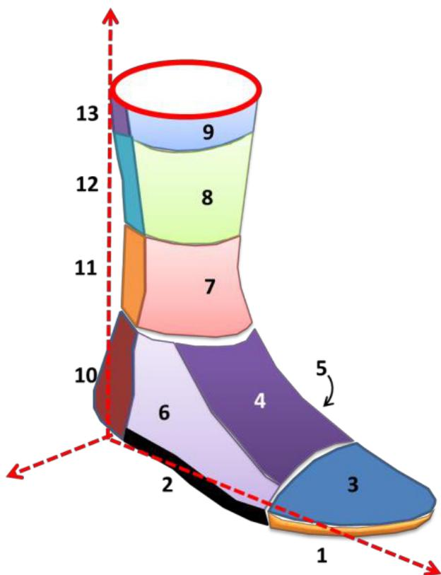
Fig. 3 Thermal foot manikin divided into 13 segments [23]
