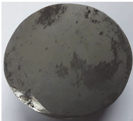
Figure 11 Cross-section of the flotation ball
