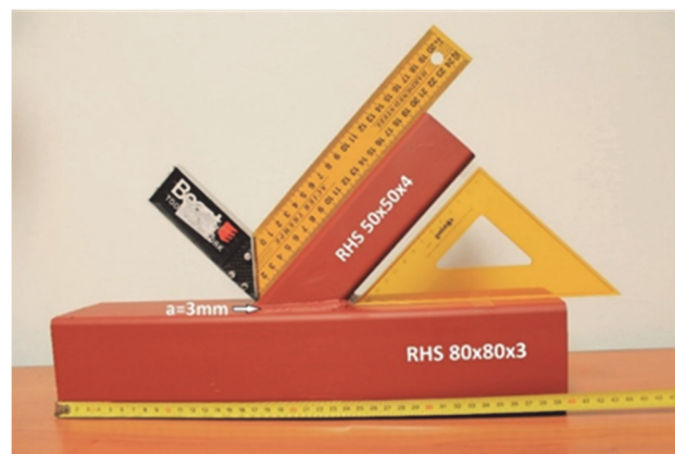
Figure 1 Geometry of Y-joint samples
