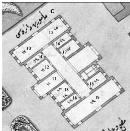
FIG. 13 ADMINISTRATIVE BUILDING GROUND FLOOR PLAN: C – ADMINISTRATIVE OFFICES, 11 – INNER COURTYARD, 12 – ROOM FOR PRISONERS OF HIGHER SOCIAL STANDING, 13 – GENDARMERIE OFFICER ROOM, 14 – GENDARMERIE OFFICERS' BEDROOM, 15 – WARD FOR POLICES, 16 – INTERROGATION ROOM, 17 – SMALL KITCHEN, 18 – ISOLATION CELL, 19 – WARD FOR 30 PRISONERS
