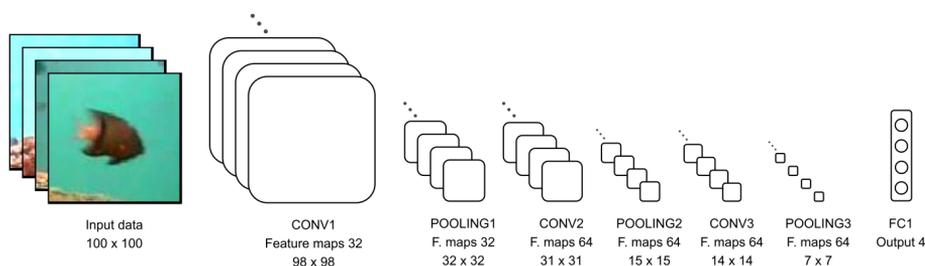
*Figure 2 – CNN architecture for fish species classification (CONV1 – first convolutional layer with 32 feature maps, POOLING1 – first pooling layer with 32 feature maps, CONV2 – second convolutional layer with 64 feature maps, POOLING2 – second pooling layer with 64 feature maps, CONV3 – third convolutional layer with 64 feature maps, POOLING3 – third pooling layer with 64 feature maps, FC1 – output layer with one neuron for each class, four classes in total)*
