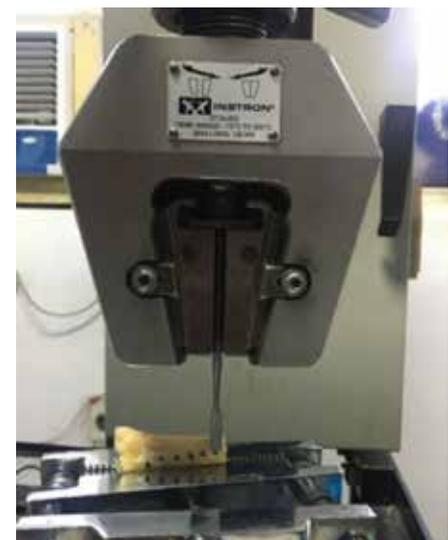
Figure 3. Universal Testing machine (Instron model 8800 MK3305 – Servo-Hydraulic)
